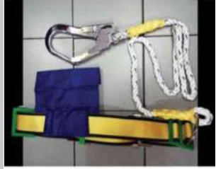
Safety belt The person will last for about 90 seconds, then the belt will be pulled tightly to the wearer's diaphragm, causing poor blood flow and possibly unconsciousness.
